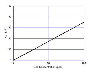
Fig. 4 - Typical sensitivity characteristics of FECS50-100
