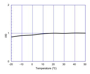
Fig. 7 - Temperature dependency (Io=sensor output current at 20°C)
