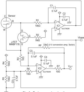
Fig. 1 - Basic measuring circuit
