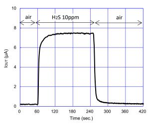
Fig. 5 - Response to hydrogen sulfide of FECS50-100
