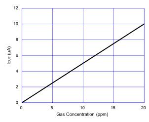
Fig. 4 - Typical sensitivity characteristics of FECS43-20
