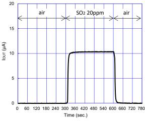
Fig. 5 - Response to sulfur dioxide of FECS43-20
