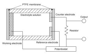
Fig. 3 - Schematic diagram of operating principle
