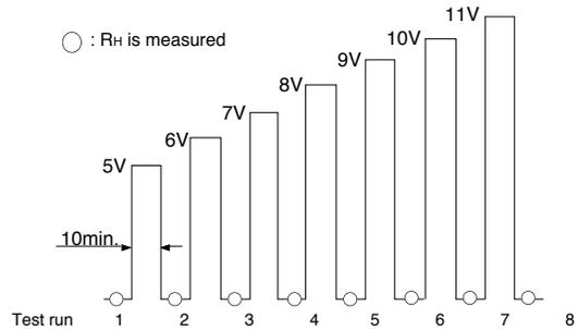
Fig. 21 - Test procedure for heater durability
