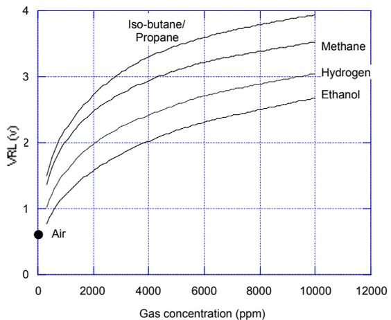
Fig. 5 - Sensitivity to various gases ( $V_{RL}$ )
