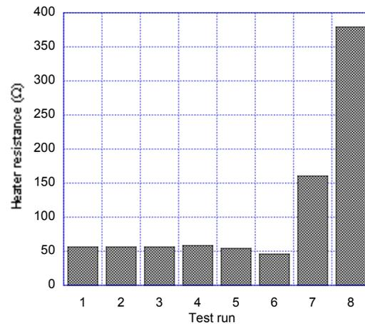
Fig. 22 - Short-term effect of  $V_H$  on  $R_H$
