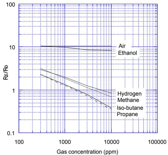
Fig. 4b - TGS2610-D00 sensitivity to various gases ( $R_s/R_o$ )
