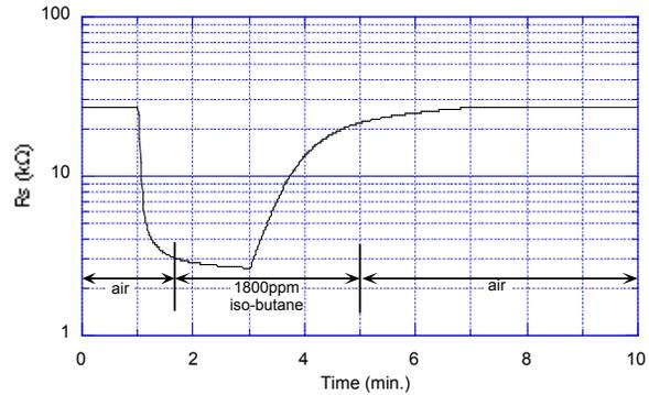
Fig. 10b - Gas response to iso-butane of TGS2610-D
