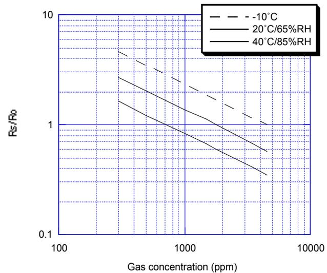
Fig. 7 - Sensor resistance under various ambient conditions
