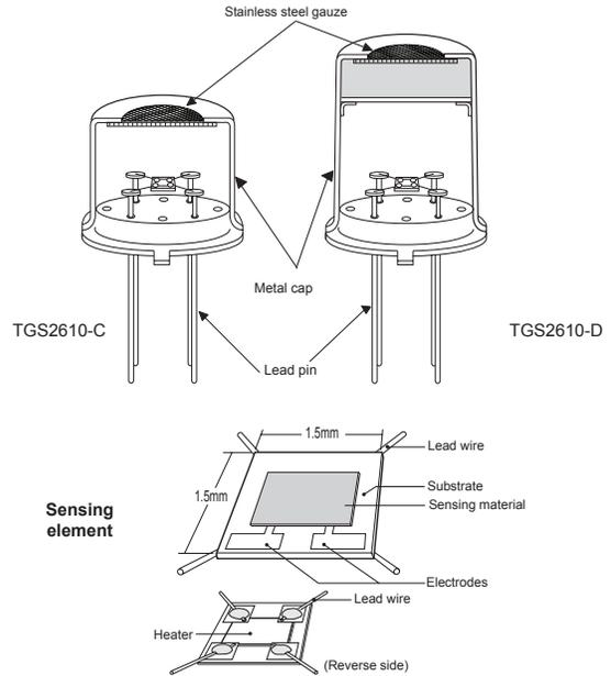
Fig. 1 - Sensor structure
