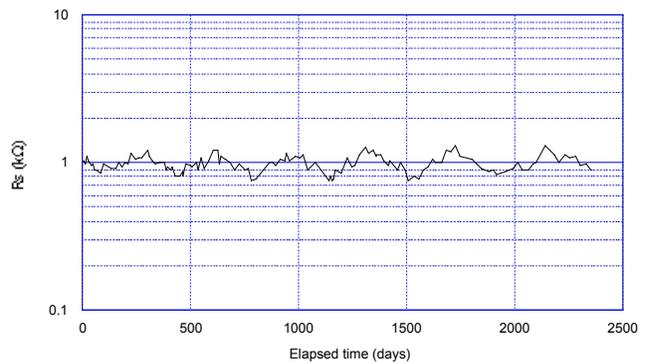
Fig. 14 - Influence of unenergizing on TGS2610-C
