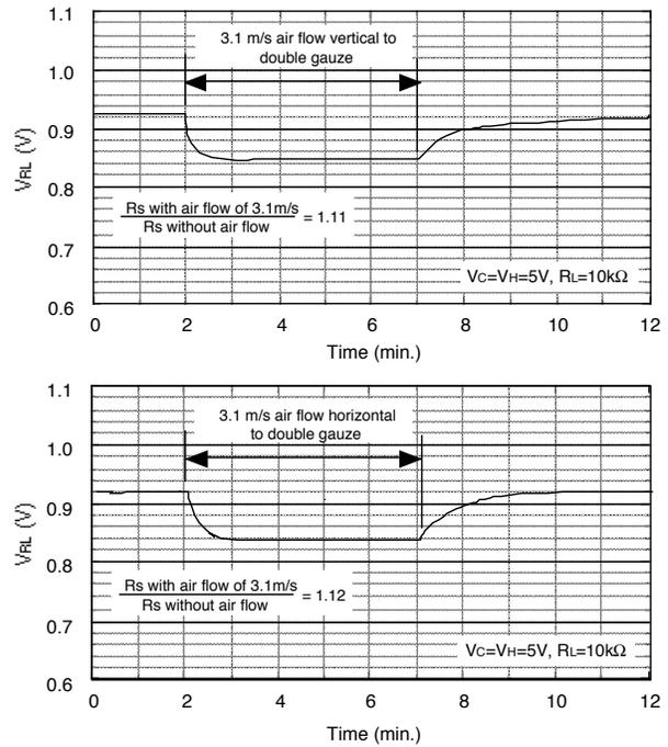
Fig. 20 - Effect of air flow on TGS2610-C
