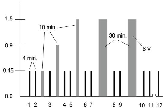
Fig. 15 - Test procedure for gas exposure
