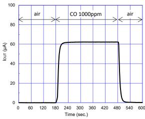
Fig. 5 - Response to carbon monoxide of FECS40-1000
