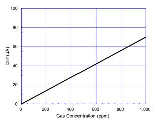
Fig. 4 - Typical sensitivity characteristics of FECS40-1000
