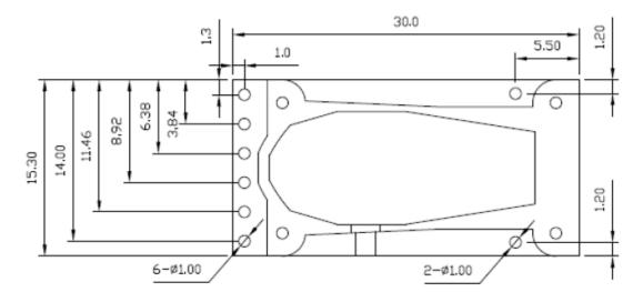
\* Module Total Dimension: 30.0mm (W) x 15.3mm (L) x 7.7mm (H)
