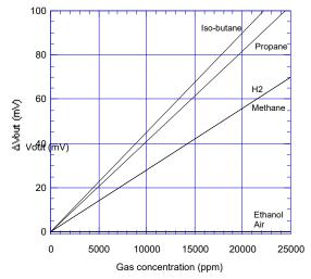
Fig. 4 - Sensitivity to various gases
