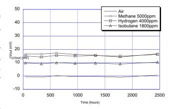
Fig. 12 - Durability to SO<sub>2</sub>
