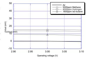
Fig. 7 - Heater voltage dependency
