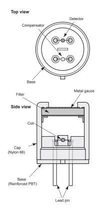
Fig. 1 - Sensor structure
