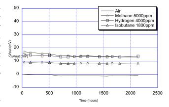
Fig. 11 - Durability to hydrogen
