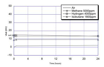
Fig. 14 - Durability to HMDS
