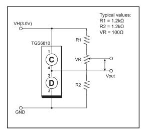
Fig. 2 - Basic measuring circuit
