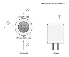
Fig. 15 - Air flow testing direction (ref. Table 1)
