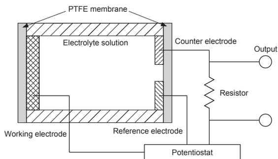
Fig. 3 - Schematic diagram of operating principle
