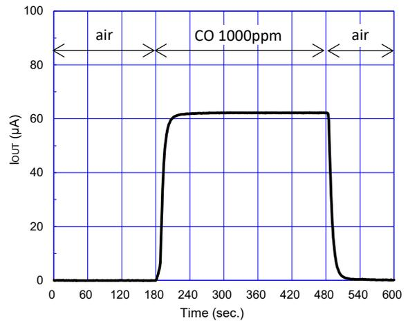
Fig. 5 - Response to carbon monoxide of FECS40-1000
