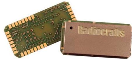
The module includes ICI, the intelligent C-programmable I/O, along with all necessary drivers and operating system. ICI allows the user to program his own intelligent sensor/actuator interface, or any other application with minimal effort. The programming capability of the module makes it possible to interface to any sensor/actuator or combination of sensors/actuators, thereby removing the need for an additional MCU to reduce overall cost and power consumption.
