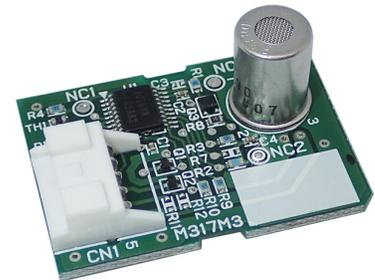
\* FCM Series is the model name of refrigerant gas sensor modules supplied by Figaro Engineering Inc.
