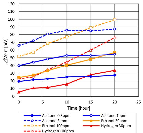
Fig.14b - Influence of OMCTS exposure on the output voltage difference  $\Delta V_{\text{OUT}}$  in acetone, ethanol and hydrogen.
