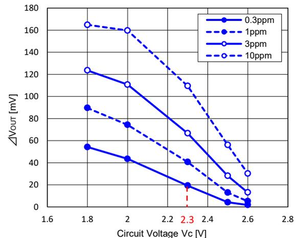
Fig. 7b - Circuit voltage dependency of sensitivity to Acetone  $\Delta V_{OUT}$
