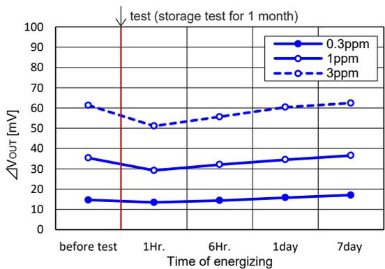
Fig.15b - Effect of storage at 20°C, 65%RH on the sensitivity to acetone  $\Delta V_{\text{OUT}}$
