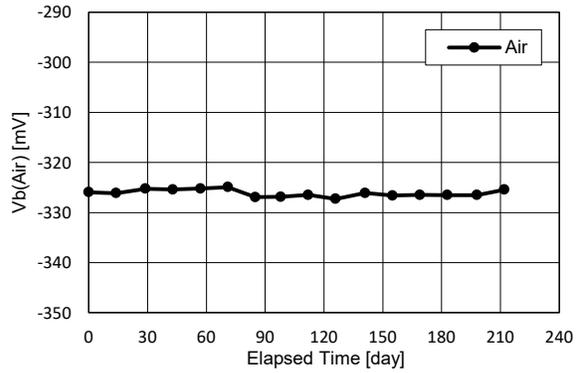
Fig. 11a - Long term stability of the sensor output in air ( $V_b(\text{Air})$ ) in unenergized condition
