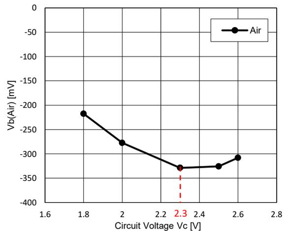
Fig. 7a - Circuit voltage dependency in Air  $V_b(\text{Air})$
