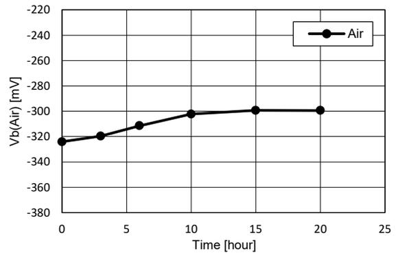
Fig.14a - Influence of OMCTS exposure on sensor output voltage  $V_b(\text{air})$
