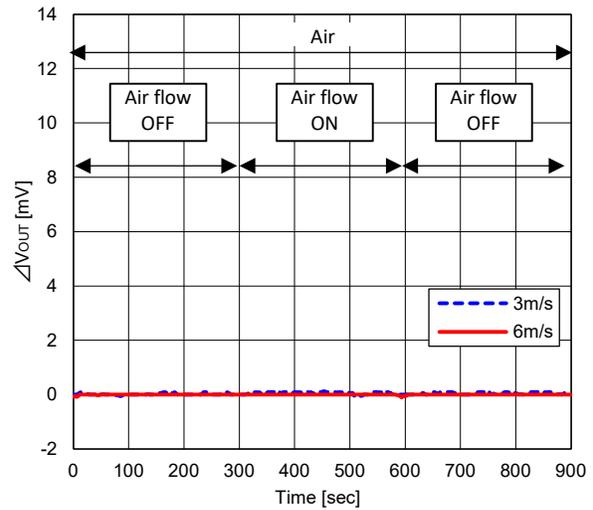
Fig. 12a - Effect of air flow in Air  $\Delta V_{OUT}$
