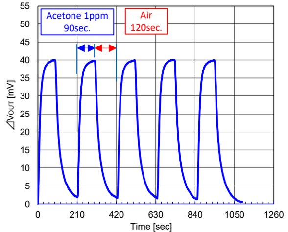
Fig. 6 - Repeatability of sensor output  $\Delta V_{OUT}$  (1ppm of Acetone)
