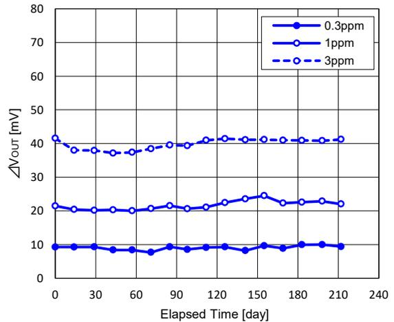
Fig. 11b - Long term stability of sensitivity to acetone ( $\Delta V_{\text{OUT}}$ ) in unenergized condition
