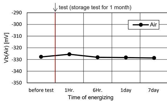
Fig.15c - Effect of storage at 40°C, 85%RH on the sensor output in air  $V_b(\text{Air})$
