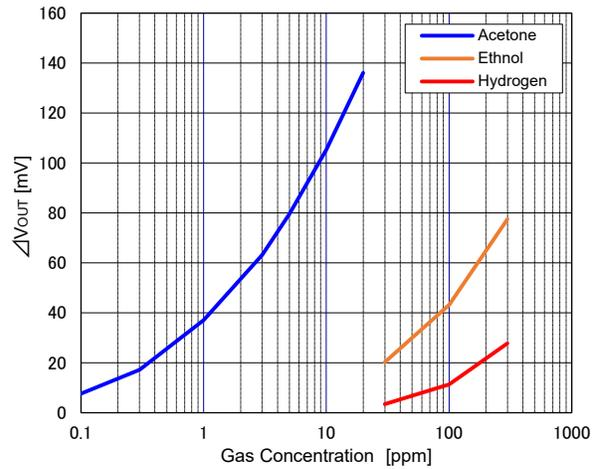
Fig. 4 - Sensitivity to acetone, ethanol and hydrogen ( $\Delta V_{OUT}$ )
