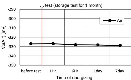
Fig.15a - Effect of storage at 20°C, 65%RH on the sensor output in air  $V_b(\text{Air})$
