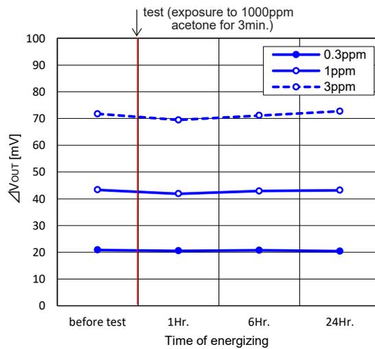
Fig.13b - Effect of exposure to high concentration acetone on sensitivity to acetone  $\Delta V_{\text{OUT}}$
