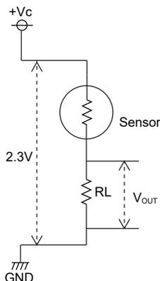
Measure the voltage ( $V_{OUT}$ ) across the load resistor  $R_L$ .  $\Delta V_{OUT}$  can be calculated by the following formula.
