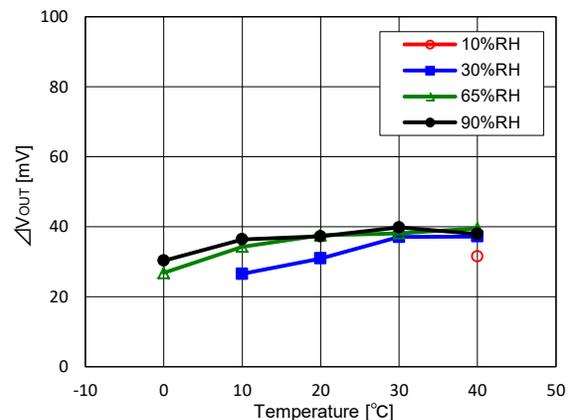
Fig. 5b - Temperature and humidity dependency of sensitivity to 1ppm Acetone
