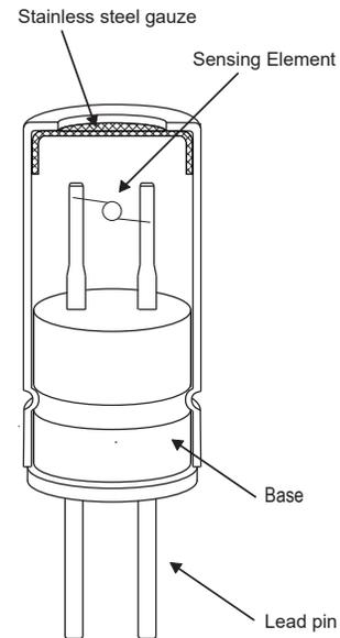
Fig. 1 - Sensor structure
