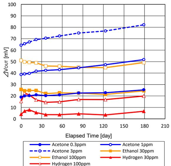
Fig. 10b - Long term stability of sensitivity to acetone, ethanol and hydrogen ( $\Delta V_{\text{OUT}}$ )
