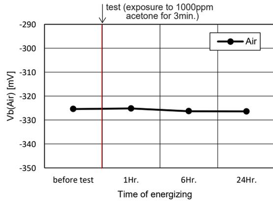
Fig.13a - Effect of exposure to high concentration acetone on sensor output in Air  $V_b(\text{Air})$
