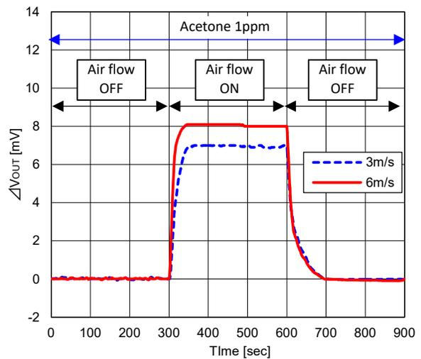
Fig. 12b - Effect of air flow in 1ppm acetone  $\Delta V_{OUT}$
