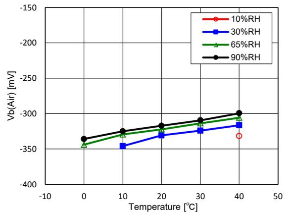
Fig. 5a - Temperature and humidity dependency in clean air ( $V_b$ )
