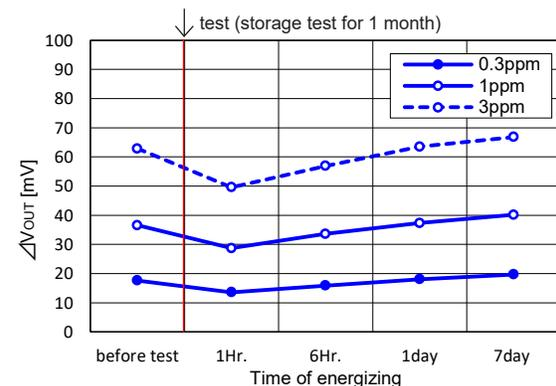
Fig.15d - Effect of storage at 40°C, 85%RH on the sensitivity to acetone  $\Delta V_{\text{OUT}}$
