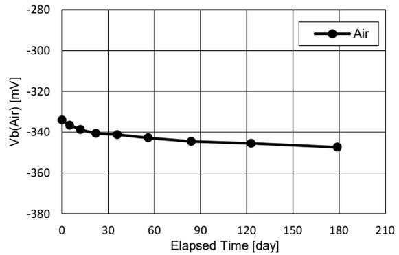
Fig. 10a - Long term stability of the sensor output in air ( $V_b(\text{Air})$ )
