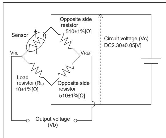
Fig. 2 - Basic measuring circuit
