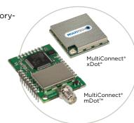
The mDot and xDot are LoRaWAN compliant,
