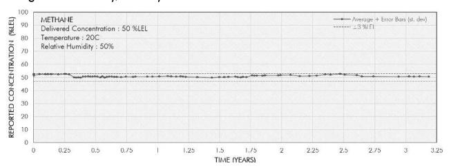
Average concentration reported to repeated exposures of 50 %LEL methane vs. time. Between exposures, all sensors were operated without airflow in ambient air. During exposures, all sensors were placed in an environmental chamber set at standard conditions (20 °C, 50 %RH) where gas was delivered from a cylinder. Accuracy remains within  $\pm 3$  %LEL over 3 years.
