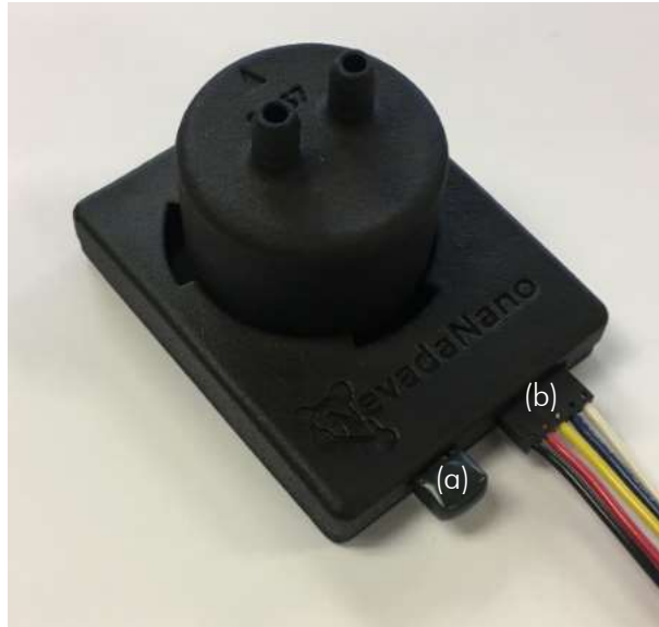
Figure 10 – Alternative communication configuration. The micro USB plug (a) is inserted prior to interfacing with the sensor via the 5-pin header (b)
