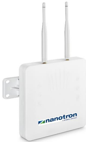
Figure 2 nanoANQ EA housing with antennas
